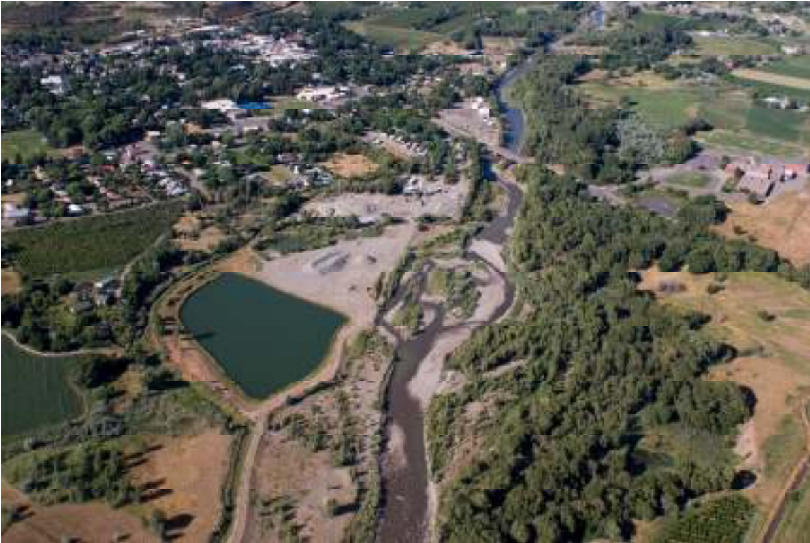
Paonia River Park: Historic in-stream gravel mining, channel incision, bank erosion, braided stream channel, annual flooding
